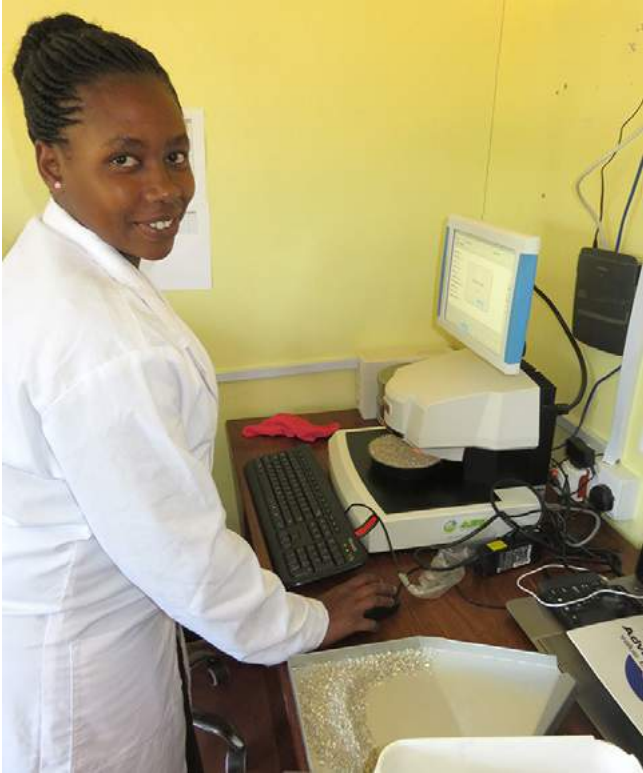
Checking feed composition with a near-infrared spectroscopy machine.
