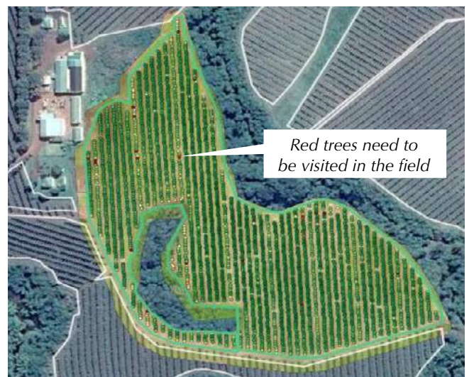
Plant health is assessed using imagery showing Normalised Difference Vegetation Index (NDVI) values. These help management efficiently grow the most uniform and productive crop. Imagery can be useful at a broad scale (left) or to monitor individual trees in an orchard (right).
